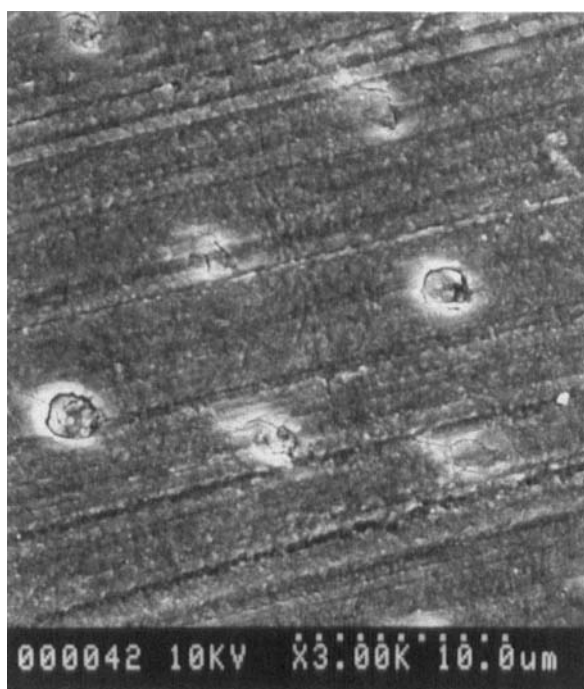
FIGURE 8 Surface of ground dentin treated with PENTA/HEMA (SEM, 3,000 \times ). A layer largely obliterating tubules remains on the surface.
