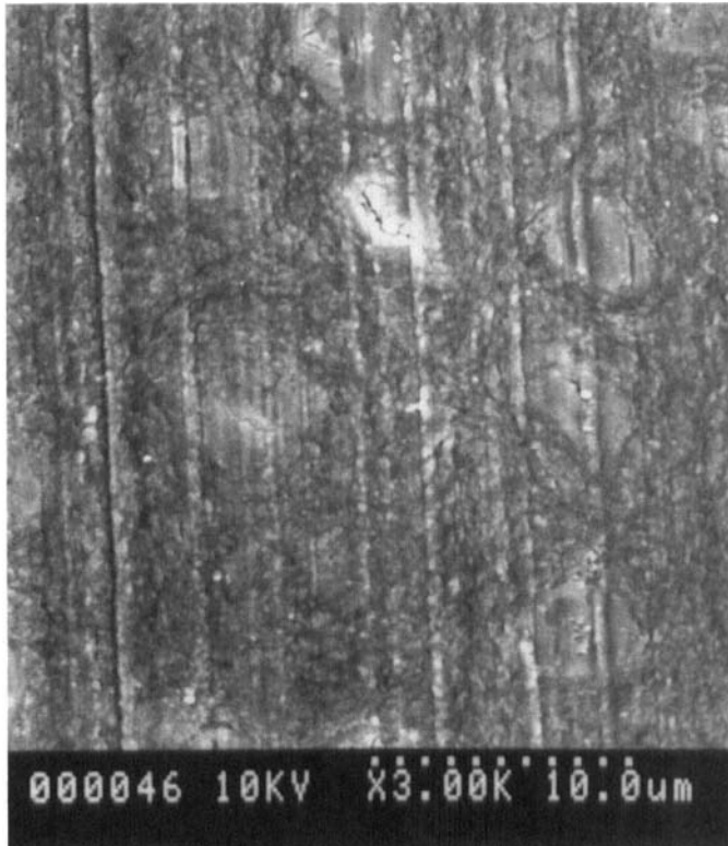
FIGURE 2 Surface of ground dentin showing smear layer covering surface (viewed by scanning electron microscopy, 3,000 ×).
